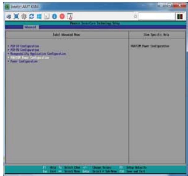
4. To enable the power, select COM1, COM2 or COM3 Power setting and press <Enter>. Select Power and press <Enter>. Save the change by pressing F10.
