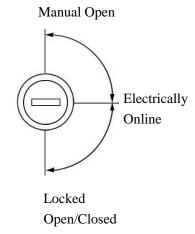
Warning: To reduce the risk of damaging or breaking the key, avoid leaving it in the lock during normal operation
