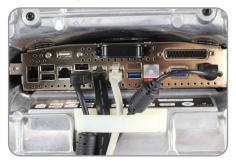
Run all cables through the cable clip on the base and out the back for optimal cable management.
