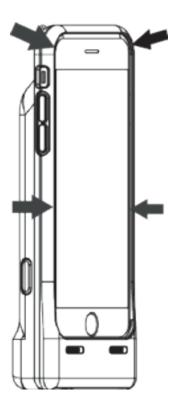
4. To remove the iPhone, bend the top corners of the jacket. Place your finger in between the jacket and the iPhone, and pull the iPhone up and out of the jacket. Be careful not to damage the lighting connector at the bottom of the jacket.
