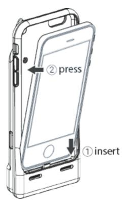
3. Take the unit and snap the top corners into the jacket. Double check the sides and corners to make sure everything is in place and secured.
