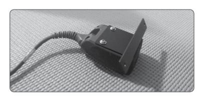
Place your POS-X TP4 Face down on a soft material to avoid scratches. Remove the two middlemost screws from the bottom of the back of the screen
